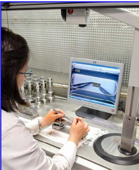
The matching of strain gauge characteristics to those of the load measuring element is crucial, especially where creep and linearity characteristics are concerned. The performance of the finished load cell is also directly dependent on the repeatable nature of the strain gauge bonding process.
